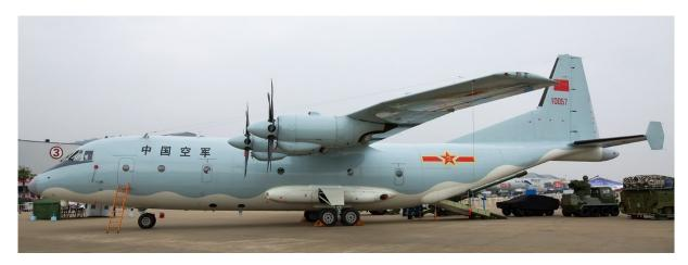
Shaanxi Y-9 multi-purpose transport, developed as a stretched version of the Shaanxi Y-8 with greater payload and range.
